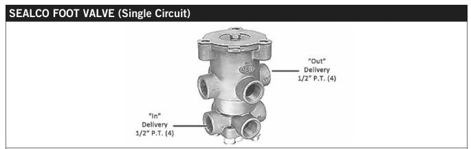
Single Circuit Foot Valve — Normally used on pre FMVSS-121 vehicles. It is foot operated and controls the delivery of air to the brake chambers. Simply stated it provides the drive with a means of applying and releasing the brakes on a vehicle.
