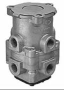
Dual Circuit Foot Valves — A dual foot has two separate circuits for service and secondary braking, and is used in dual circuit air brake systems mandated by FMVSS-121. Braking ability is maintained in the event that one circuit fails.
