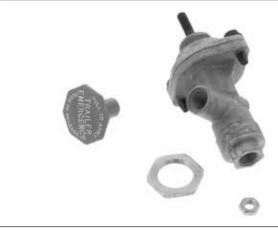
Push-Pull Valves — Manually operable — Pressure sensitive, on/off valves which will automatically return to the button out (exhaust) position when supply pressure is below the required minimum.
