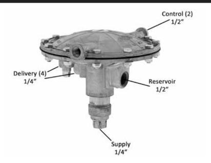
Relay Emergency Valve — A dual function valve used on trailers.
