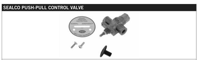
Push-Pull Valves — Manually operable — Pressure sensitive, on/off valves which will automatically return to the button out (exhaust) position when supply pressure is below the required minimum.
